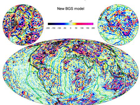
Vertical component of the BGS lithospheric magnetic field. The model is computed to spherical harmonic degree 133, resolving features down to ~300 km.
