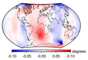
Declination differences at Earth's surface at 2016.0 between a truncated BGS model and WMM2015.
