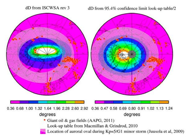
Declination standard errors from the industry error model (left) and from a BGGM look-up table (right).
