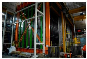
The OPERA detector at Laboratori Nazionali del Gran Sasso, which detects the neutrino beam from CERN (picture courtesy of Luca Giovanelli).
