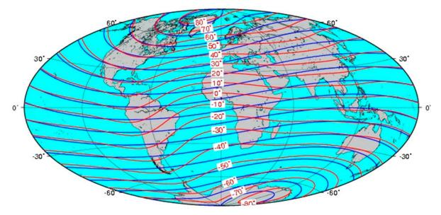
Different methods of defining geomagnetic latitude: dipole (blue) and guasi-dipolar (red) contours at 2015.0.
