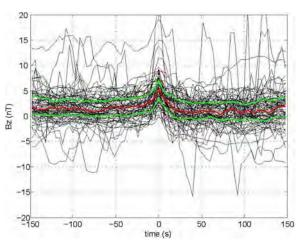
Signature of tail-ward-propagating dipolarisation fronts in the Z-component of the magnetic field in Cluster spacecraft data. Red (green) is the mean (mean +/- 1 standard deviation) level from a number of superposed events.(Nina Kahr)
