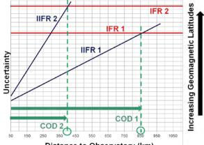
Distance to Observatory (km) Schematic to demonstrate the improvement in uncertainty using IIFR over IFR and how this drops off with distance from the drilling location. Two example geomagnetic latitudes (1=lower and 2=higher latitude) are show. The COD is reached when IIFR (blue) no longer reduces the uncertainty compared to IFR (red).
