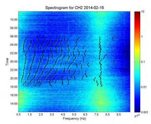
Results from the automatic detection of SRS
