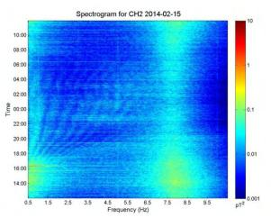
Spectrogram for 15/16<sup>th</sup> March 2014. The wispy fringes between 18:00-04:00 and 1-5 Hz are the lonospheric Alfvén Resonances. The first Schumann resonance is the diffuse region visible around 8 Hz
