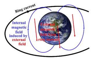
Simplified diagram of the Earth's ring current (black) and the magnetic fields it produces: external (red) and induced internal (blue)
