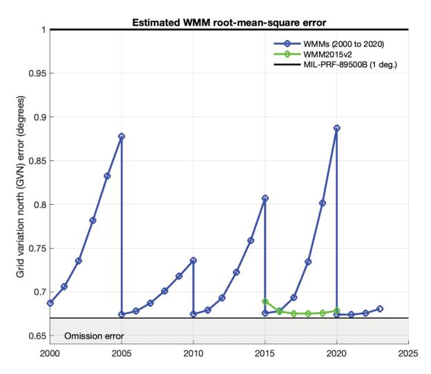
**Figure 1:** WMM global RMSE for the grid variation north (GVN) component from 2000 to 2023. Errors for six successive WMMs are shown: WMM2000, WMM2005, WMM2010, WMM2015, WMM2015v2, and WMM2020. WMM2015v2 was an out-of-cycle WMM released in late 2018 in case WMM2015 were to breach the specification before the end of the cycle. (The specification was revised in 2019 with the introduction of so-called blackout zones, see below; blackout zones are no longer considered in WMM error calculations.)
