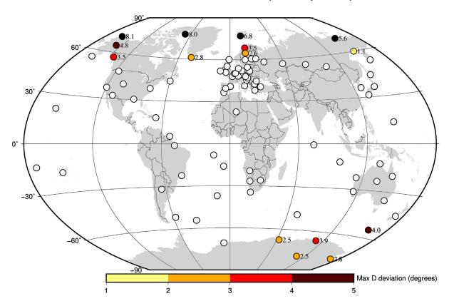
Figure 7: Indicative maximum declination deviations during G4 storm on 4 November 2021. The white circles are observatories where the maximum deviation is less than the military specification of 1°.
