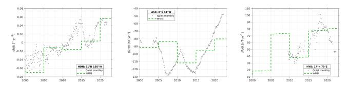
Figure 3: Observed rate of change of (a) inclination angle in degrees (I) at Honolulu, Hawai'i, United States (HON), (b) vertical field (Z) in nT/year at Ascension Island, South Atlantic (ASC) and (c) field intensity (F) in nT/year at Hyderabad, India (HYB). Quiet-dark monthly mean data are shown as gray circles, WMM predictions (WMM2000, WMM2005, WMM2010, WMM2015v2, WMM2020) are shown by the green dashed line.
