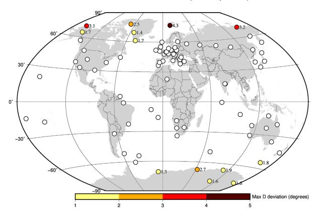
Figure 8: Indicative maximum declination deviations during G3 storm on 10 April 2022. The white circles are observatories where the maximum deviation is less than the military specification of 1°.
